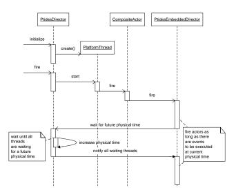
Figure 7: Simulation of a PTIDES model in Ptolemy.
