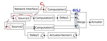
Figure 5: Distributed DE model with a sensor on one platform and an actuator on another.
