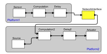
Figure 4: Distributed DE model with a sensor on one platform and an actuator on another.
